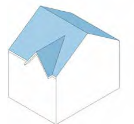
Fig 5.51 - Half gable roof
