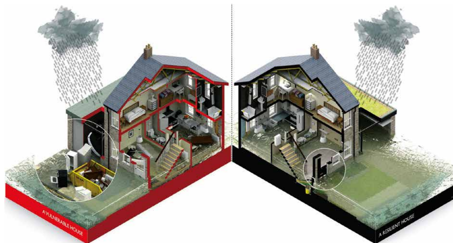
Fig 6.78 - The difference between a flood resilient house and a vulnerable house. Credit: Edward Barsley / The Environmental Studio
